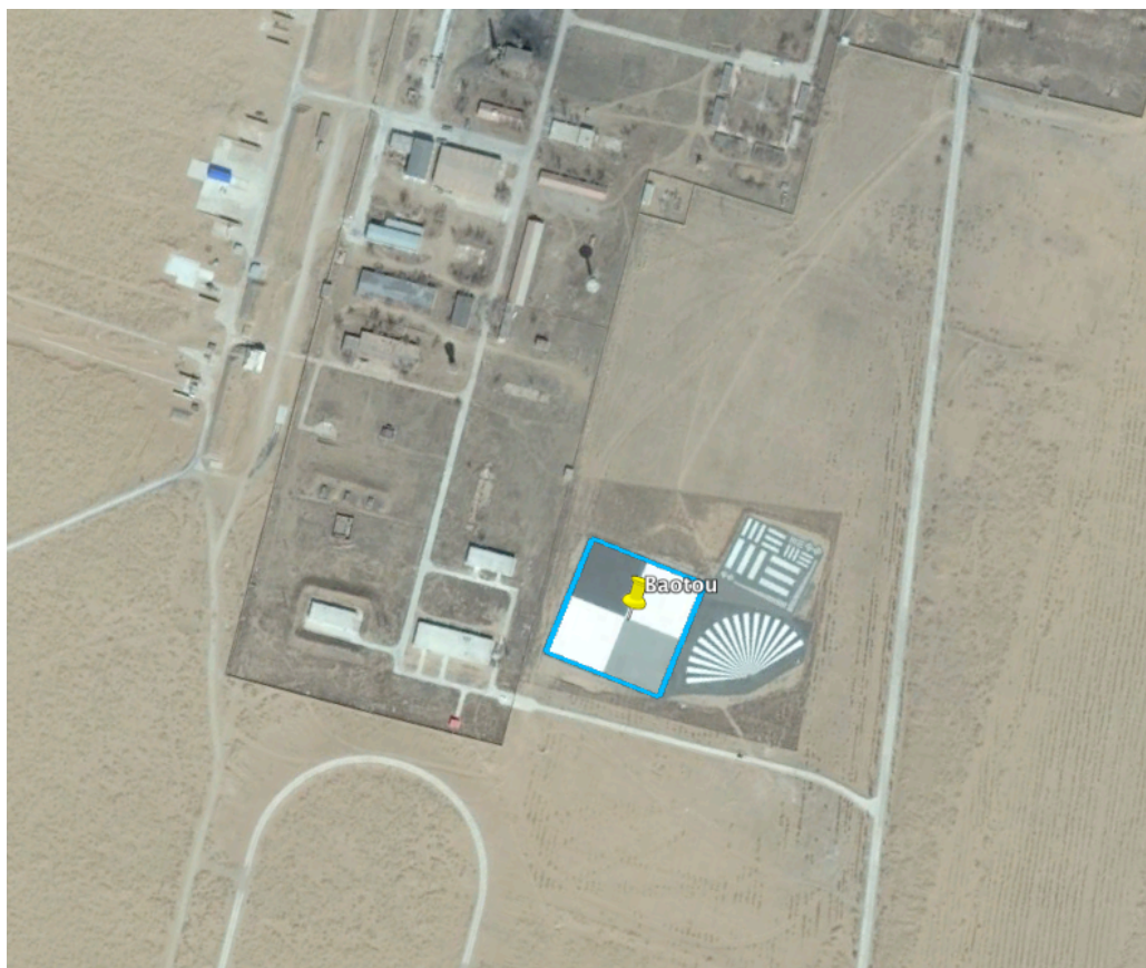
Figure 2: The Baotou artificial target highlighted in blue is composed of 4 square areas of different shades (2x white, 1 x black and 1 x grey). The RadCalNet TOA simulations are representative ONLY of the bottom right grey square within this artificial target.
